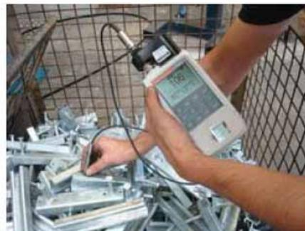
• Electronic gauge for galvanize coating thickness check
